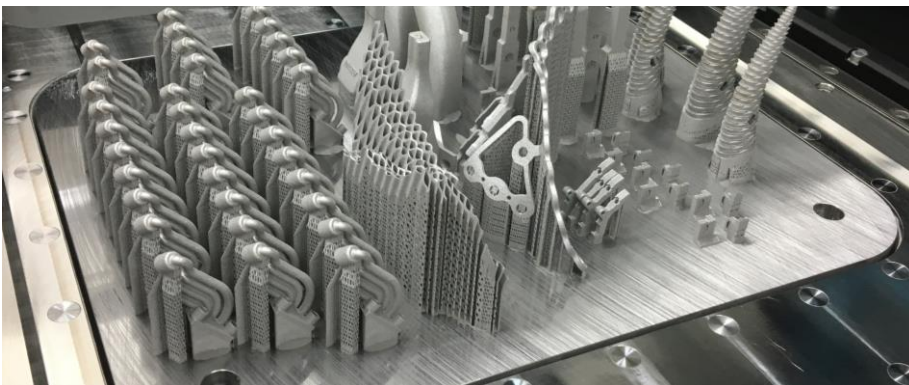
Figure 1: Chrome steel build job on a build plate of 400mm x 325mm
